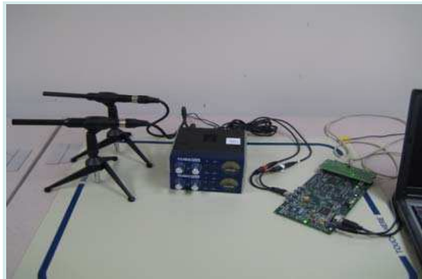
Fig. 2. The DSP-based prototype for real-time one-way communication
