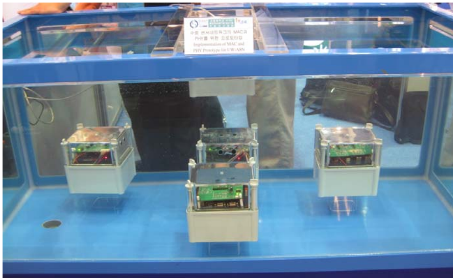
Figure 1 – Deployed underwater sensor nodes in a water tank.
